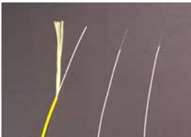
JACKET 900 MICRON 250 MICRON THREE FIBER STRIPPING STATIONS
