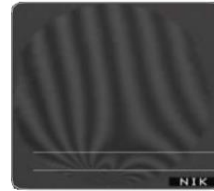
1,000 μm diameter fiber Interference microscope image 1 stripe = 0.01°
