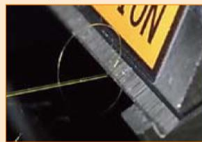
Coating is peeled off with stripping blade.
